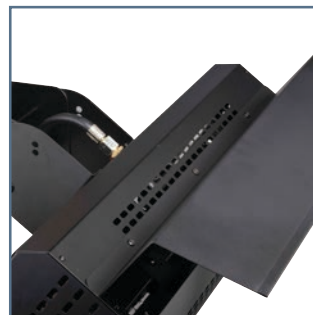
The standard heat reflector ensures only 500mm overhead clearance is required. The optional HeatShield (TGHAC-003) 0098304 reduces this to 300mm clearance.
